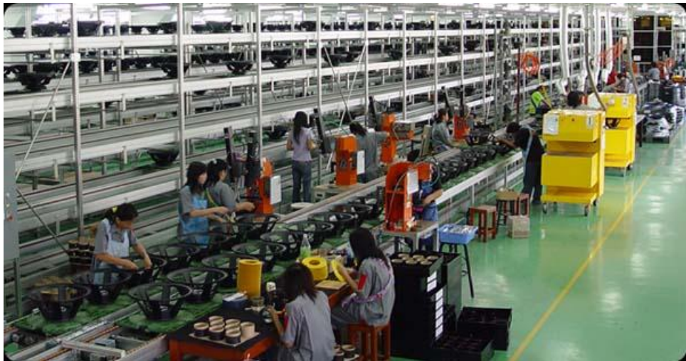
The company's 2.5 km production line can produce 4,800 woofers during three shifts per day.
