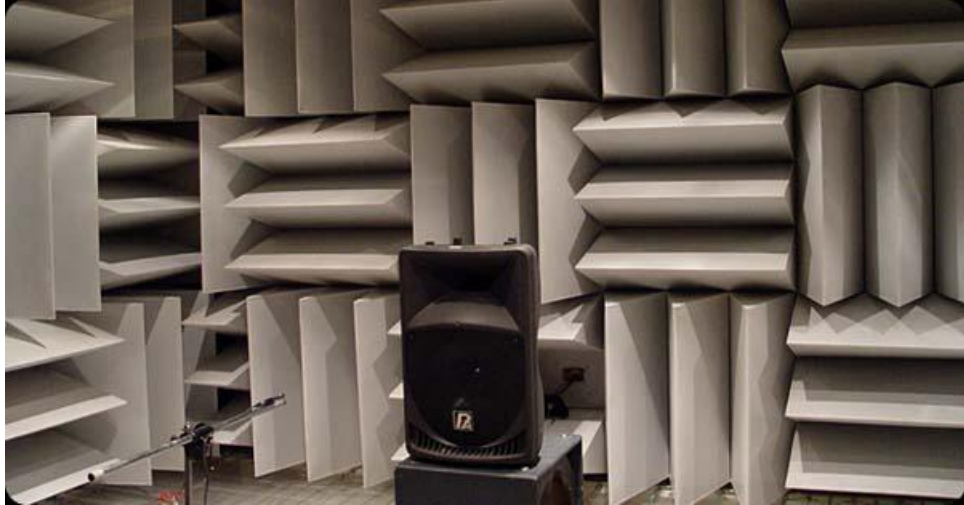
A large anechoic chamber provides an ideal environment for product evaluation and development at P.Audio System's main factory in Thailand.
